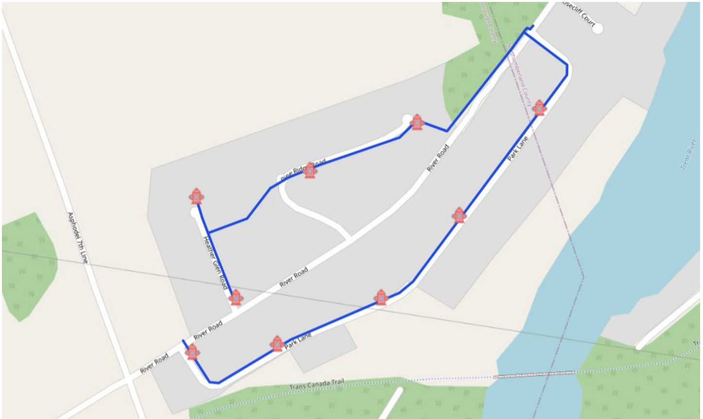
Figure 91 Trentview Estates Water Distribution and Hydrant Network
